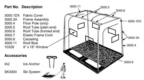
**NOTE:** Small Holes, Tears and Cuts in Cover can be Repaired with Black Duct Tape applied to Coated Side of Fabric.
